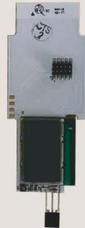
This one module, integrating Wi-Fi, Bluetooth, microprocessor, memory and an ambient light sensor, is the solution to a simple, affordable universal IoT gateway.
