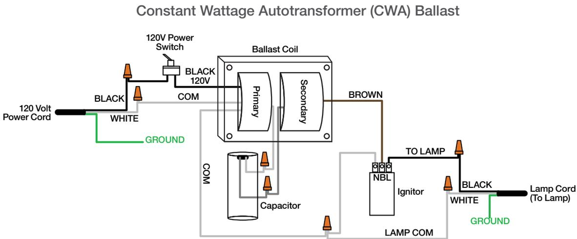
**Fig. 5** Simplified magnetic ballast architecture with compensating capacitor. An inductor is used to limit power and control current to the lamp while a capacitor is used to compensate for the lagging (inductive) load and generate a high power factor. The capacitor is sized to the relative load of the lamp.
