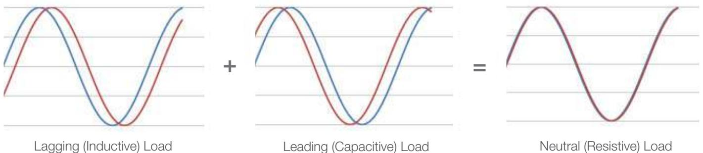
**Fig. 2** When lagging and leading loads are added together, they have the helpful effect of canceling each other out as can be seen in Fig. 2. For example a 10A load with a lagging 0.6PF and a 10A load with a leading 0.7PF when added together create a combined load of 13A with a lagging PF of 0.99.
