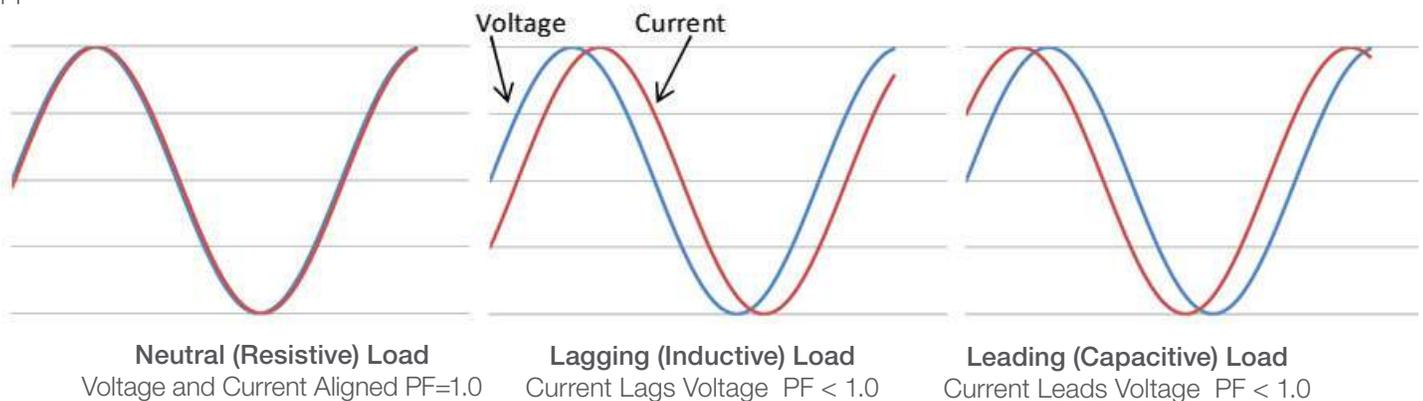
**Fig. 1** Power factor for a neutral (resistive) load vs. lagging (inductive) or leading (capacitive) loads. Loads seen in buildings are typically a combination of resistive and inductive loads driven by electric motors, magnetic ballasts and mixed plug loads.
